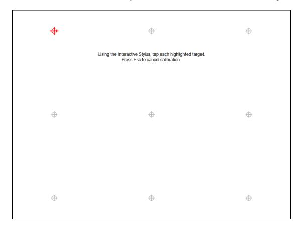
To calibrate, use the Interactive Stylus and click in the centre of each red symbol. You will hear a beep and the next symbol will turn red. When you have finished the eBeam knows where to read the data.
